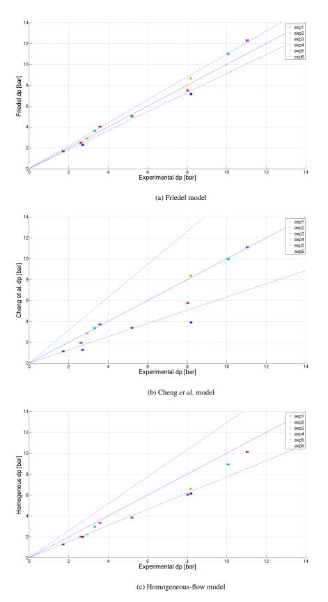
Figure 3: Comparison between experimental and calculated frictional pressure drop.
