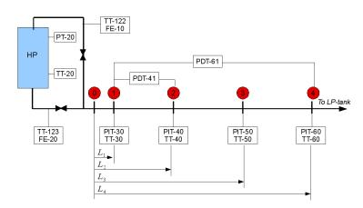
Figure 1: The test rig. Sensors measuring absolute pressure (PIT and PT), differential pressure (PDT), temperature (TT) and mass flow rates (FE) are placed as shown.  $L_1 = 0.2 \text{ m}$ ,  $L_2 = 50.5 \text{ m}$ ,  $L_3 = 101 \text{ m}$  and  $L_4 = 139 \text{ m}$ .
