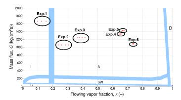
Figure 2: Flow patterns predicted by the Cheng *et al.* model for each experiment. S: Stratified, SW: Stratified-wavy, I: Intermittent, A: Annular, D: Dry-out.
