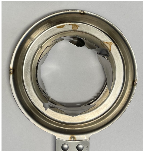
(a) Triple-layer rupture disk after test.
