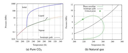
Figure 1: Isentropic depressurization from p = 12 MPa, T = 293 K. CO<sub>2</sub> is in a dense liquid state until it reaches the saturation line and then the triple point, whereas the natural gas is in a dense gaseous state until it reaches the two-phase area. The Span-Wagner EOS has been used for CO<sub>2</sub> and the Peng-Robinson EOS for natural gas. The natural gas composition is given in Table 1.
