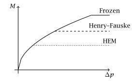
Figure 3: Illustration of the two-phase mass-flow rate M through an orifice as a function of the pressure difference  $\Delta p$ , for different equilibrium assumptions.
