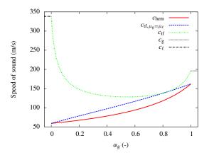
Figure 2: Speed of sound of pure CO<sub>2</sub> in the gas-liquid two-phase area as a function of gas volume fraction for various two-phase flow models. T = 250 K, SW EOS. 'hem' denotes the homogeneous equilibrium model, 'tf' denotes the two-fluid model with no phase change and no slip, 'tf  $\mu_g = \mu_\ell$ ' is the two-fluid model with full chemical equilibrium and no slip, 'g' is gas and ' $\ell$ ' is liquid.
