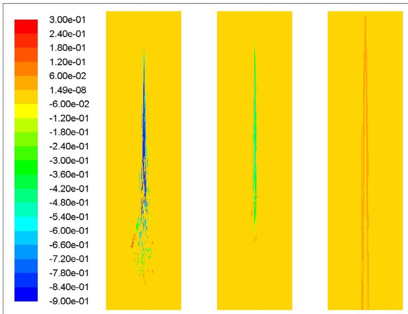
Fig. 10. Contours of relative rate differences  $(\Theta - \Theta_0)/\Theta_0$  inside the particle jet, from left to right:  $m_f = 1.5 \cdot 10^{-2}$  kg/s,  $m_f = 1.5 \cdot 10^{-3}$  kg/s and  $m_f = 1.5 \cdot 10^{-4}$  kg/s.
