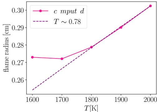
Figure 7: Effective flame radius in a function of temperature
