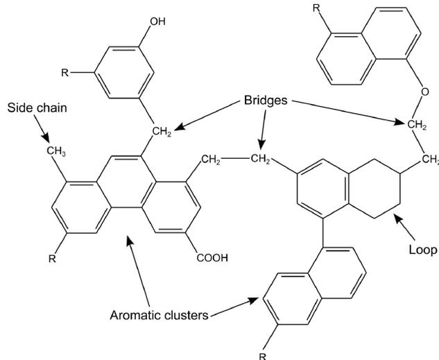
**Figure 1.4:** Schematics of the coal chemical structure (reused from [3] based on CC-BY license). From the chemical standpoint, coal consists of organic matrix with mineral inclusions. The organic part, shown in the figure, is a macromolecular network composed of condensed aromatic rings and peripheral groups (side chains). The rings are grouped into aromatic nuclei (clusters) that are connected with each other by labile bridges [4].
