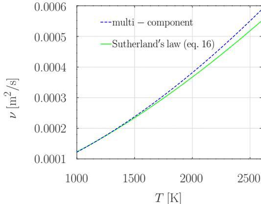
Figure 1: Kinetic viscosity as obtained using Sutherland’s law (Eq. (16)) and multi-component approach for the mixture consisting of  $Y_{N_2} = 0.7292$ ,  $Y_{O_2} = 0.05$ ,  $Y_{H_2O} = 0.0008$ ,  $Y_{CO} = 0.02$  and  $Y_{CO_2} = 0.2$
