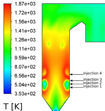
Fig. 14. Contours of temperature in the boiler central cross section. Arrows indicate elevations of fuel injection ports.
