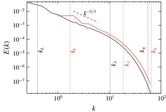
FIGURE 1. (Colour online) Kinetic energy spectrum; black:  $Re_\lambda \approx 350$ , red:  $Re_\lambda \approx 150$  (cases A and M in table 1). The wavenumbers  $k_L$ ,  $k_\lambda$  and  $k_\eta$  correspond to the integral, Taylor and Kolmogorov scales, respectively.
