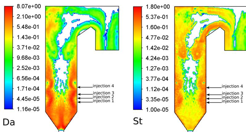
**Figure 3.2:** Distribution of Damköhler and Stokes numbers inside the investigated practical system (figure reproduced from [1]). The strongest effect of particle clustering is expected to be observed at high  $Da$  and at  $St \sim 0.1$  (in lower parts of the boiler and around injections), while the effect associated with relative velocity is expected to be most pronounced at relatively low  $Da$ , in the upper part of the domain. White areas are regions with no particles.
