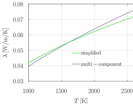
Figure 2: Thermal conductivity as obtained using Eq. (17) with  $\text{Pr} = 0.9$  and multi-component approach for the mixture consisting of  $Y_{\text{N}_2} = 0.7292$ ,  $Y_{\text{O}_2} = 0.05$ ,  $Y_{\text{H}_2\text{O}} = 0.0008$ ,  $Y_{\text{CO}} = 0.02$  and  $Y_{\text{CO}_2} = 0.2$
