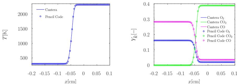
**Figure 2.2:** Comparison of 1D profiles of temperature (left) and species mass fractions (right)
