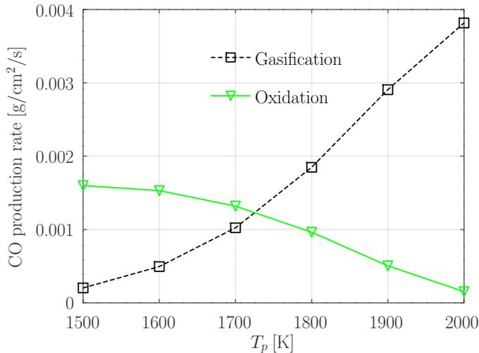
Figure 8: Contributions to CO production from gasification and oxidation
