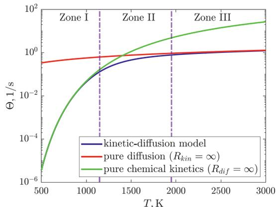
Fig. 1. The kinetic-diffusion model for  $T_p = T$ ,  $\rho_p = 800 \text{ kg/m}^3$ ,  $d_p = 500 \text{ }\mu\text{m}$ ,  $A = 0.002 \text{ s/m}$ ,  $E = 79 \text{ kJ/mol}$ ,  $C = 5 \cdot 10^{-12} \text{ sK}^{-3/4}$ .
