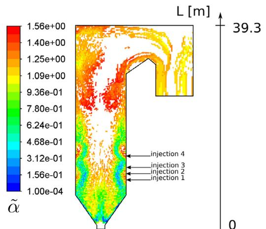
Fig. 18. Distribution of  $\tilde{\alpha}$  in the boiler central cross section. Arrows indicate elevations of fuel injection ports.
