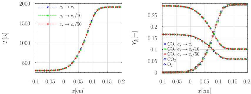
Figure 4: Comparison of temperature and species profiles across the flame obtained before and after the speed of sound reduction
