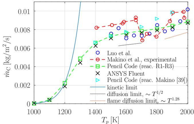
Figure 6: Comparison of carbon conversion rates as a function of particle surface temperature. The results for Luo et al. [6] are reproduced from their Fig. 8.
