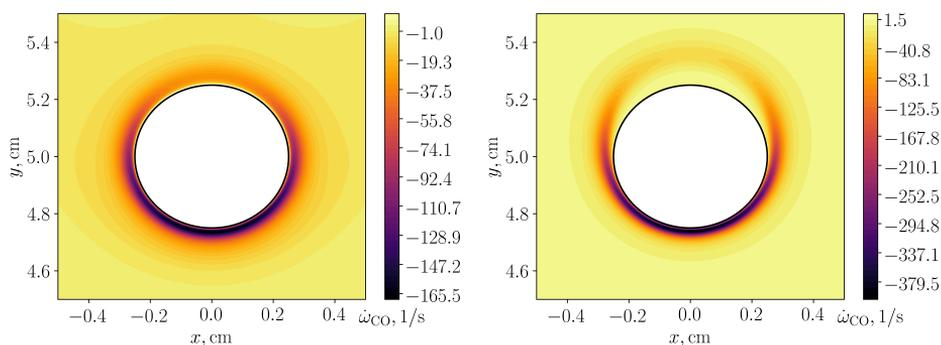
**Figure 3.3:** Contours of carbon monoxide flame, left: gas phase reaction rate reduced by a factor of 2, right: gas phase reaction rate increased by a factor of 2
