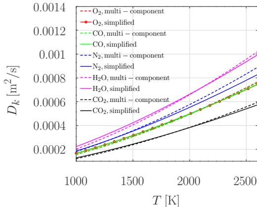
Figure 3: Diffusion coefficients as obtained using Eq. (17) (referred to as 'simplified') and multi-component approach for the mixture consisting of  $Y_{N_2} = 0.7292$ ,  $Y_{O_2} = 0.05$ ,  $Y_{H_2O} = 0.0008$ ,  $Y_{CO} = 0.02$  and  $Y_{CO_2} = 0.2$
