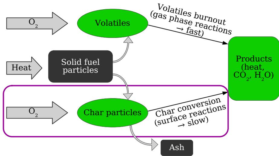
**Figure 1.3:** Schematics of the solid fuel conversion process. The focus of this thesis is on the char particle combustion, indicated in the violet frame.
