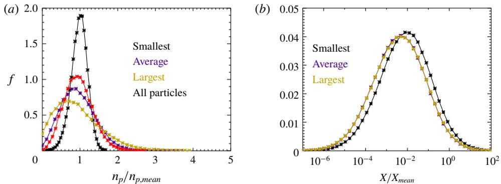
FIGURE 10. (Colour online) The p.d.f.s of (a)  $n_p/\bar{n}_p$  and (b)  $X/\bar{X}$  for different particle sizes,  $Re_\lambda \approx 350$ , compensated distr., with back-reaction,  $\bar{St}_L = 0.04$ ,  $Da = 25$  (case N).
