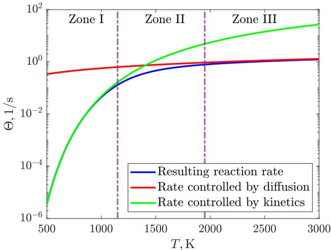
**Figure 1.5:** Combustion zones/regimes (figure reproduced basen on Fig. 1 in [1])
