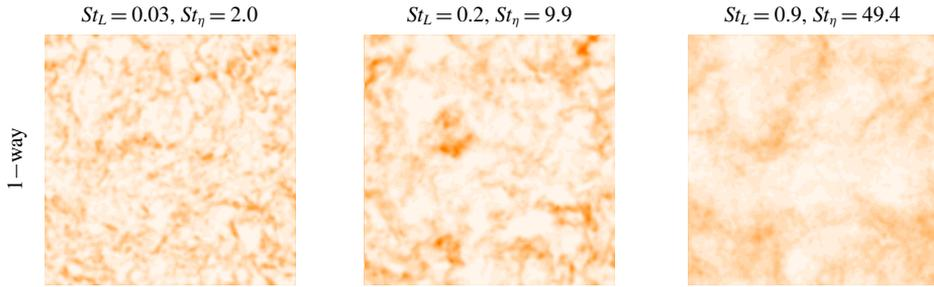
FIGURE 6. (Colour online) Particle number density for different Stokes numbers (case Q), one-way coupling,  $Re_\lambda \approx 350$ .
