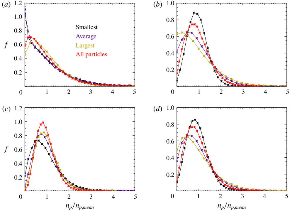
FIGURE 8. (Colour online) The p.d.f. of  $n_p/\bar{n}_p$  for different particle sizes,  $Re_\lambda \approx 150$ , compensated distr., (a,b) with back-reaction, (c,d) no back-reaction, (a,c)  $\overline{St}_L = 1.2$ , (b,d)  $\overline{St}_L = 0.05$ , in all cases  $Da \approx 35$  (cases C and F).
