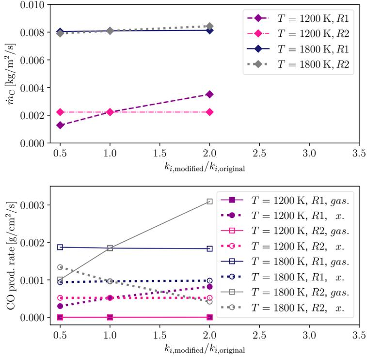
Figure 11: upper: conversion rates as obtained for modified surface reaction rates, lower: contributions from gasification/oxidation to the CO production rate. *R1* and *R2* denote oxidation and gasification, respectively, and indicate which reaction has been modified, while *ox.* and *gas.* denote contribution from oxidation and gasification to the CO production rate.
