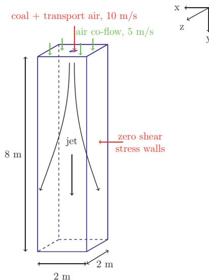
**Fig. 6.** Schematics of the geometry and boundary conditions.
