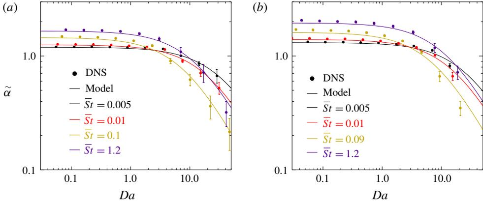
FIGURE 11. (Colour online) Normalised decay rate as a function of Damköhler number obtained for different  $\overline{St}_L$  using a compensated distribution for (a)  $Re_\lambda \approx 150$  (cases A, B, D, F) and (b)  $Re_\lambda \approx 350$  (cases L, M, O, P).
