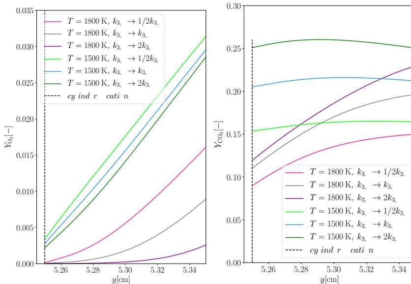
Figure 14: Oxygen and carbon dioxide mass fraction profiles along the centerline behind the particle as obtained for different gas phase reaction rates
