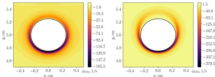
Figure 13: CO flame contours,  $T_p = 1800$  K, left:  $k_{3,f} \rightarrow 0.5k_{3,f}$ , right:  $k_{3,f} \rightarrow 2k_{3,f}$
