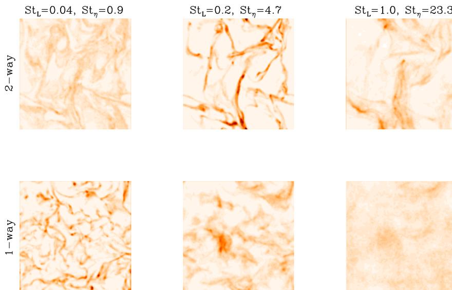
**Figure 3.1:** Particle number density for different particle sizes. The particle size grows from left to right. Upper row: 2-way coupling, lower row: 1-way coupling (figure reproduced from [2])
