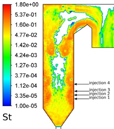
Fig. 15. Contours of the Stokes number. Arrows indicate elevations of fuel injection ports.
