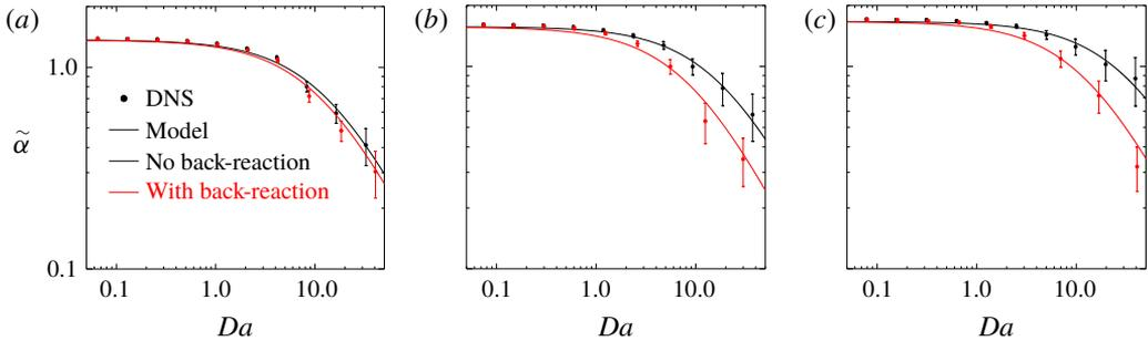
FIGURE 4. (Colour online) Comparison of the normalised decay rate obtained with and without particle back-reaction for simulations with  $\overline{St}_L = 0.05$  (a),  $0.35$  (b) and  $1.2$  (c) (cases C, E, F).
