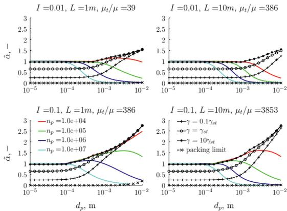
Fig. 4. The influence of parameters from Table 2 on  $\bar{\alpha}$  for char particles in air ( $\rho_p = 800 \text{ kg/m}^3$ ,  $\gamma_{st} = 11.4$ ). The legend included in the bottom panels apply to the entire figure.
