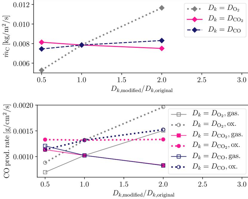
Figure 9: Upper: conversion rates for different diffusion coefficients, lower: contributions from gasification/oxidation to the CO production rate,  $T_p = 1700$  K
