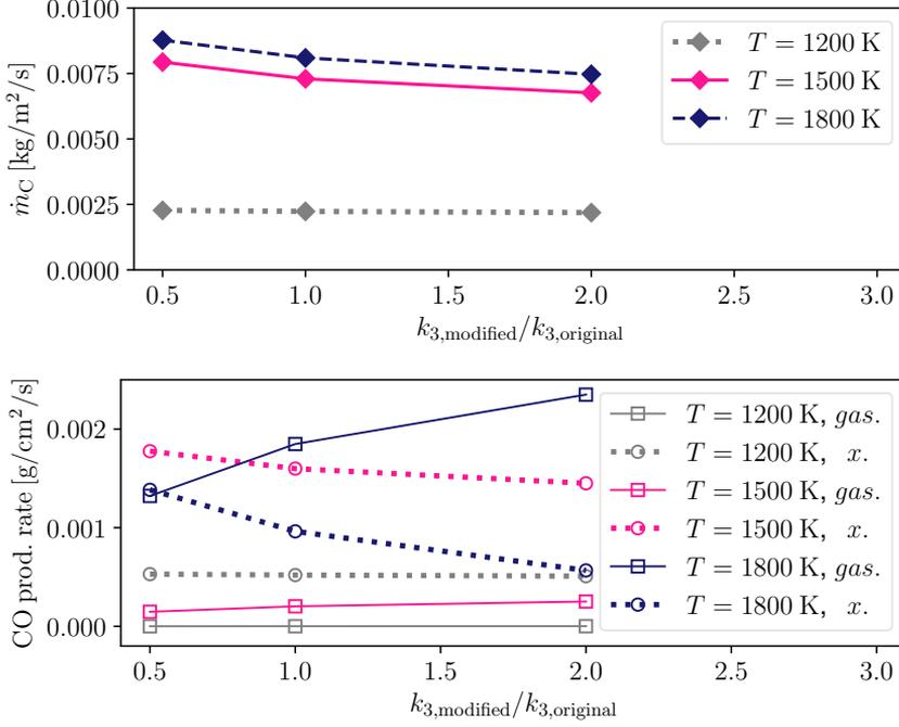
Figure 12: upper: conversion rates as obtained for modified homogeneous reaction rate, lower: contributions from gasification/oxidation to the CO production rate
