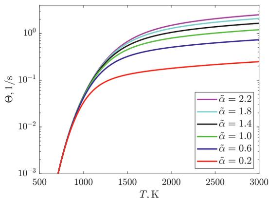
**Fig. 5.** The influence of  $\tilde{\alpha}$  on the reactant consumption rate for  $\rho_p = 800 \text{ kg/m}^3$ ,  $d_p = 500 \text{ }\mu\text{m}$ ,  $A = 0.002 \text{ s/m}$ ,  $E = 79 \text{ kJ/mol}$ ,  $C = 5 \cdot 10^{-12} \text{ sK}^{-3/4}$ .
