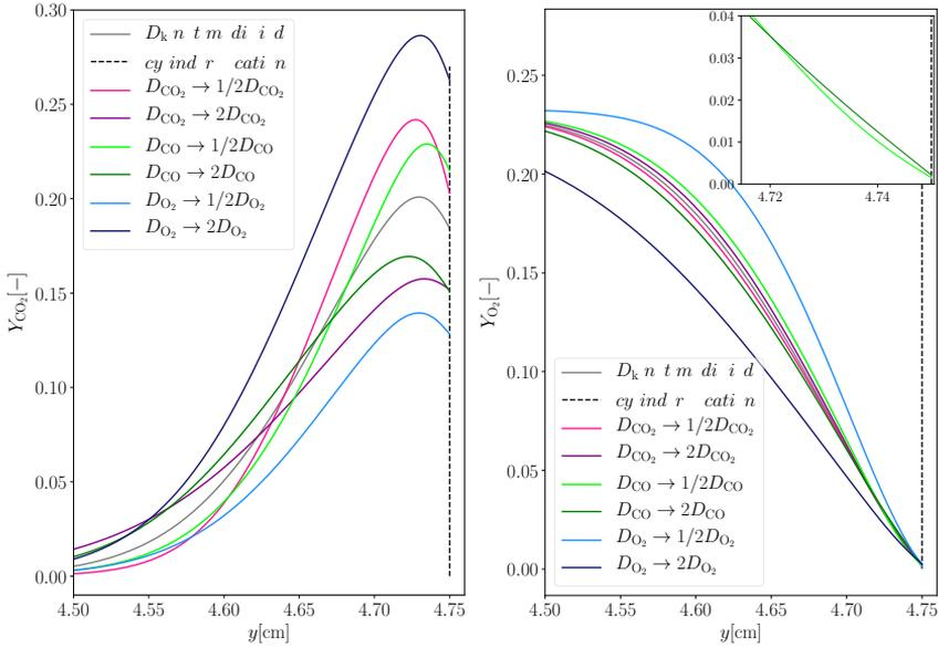
Figure 10: Oxygen and carbon dioxide mass fractions and temperature profiles in the particle stagnation region as obtained for different diffusion coefficients
