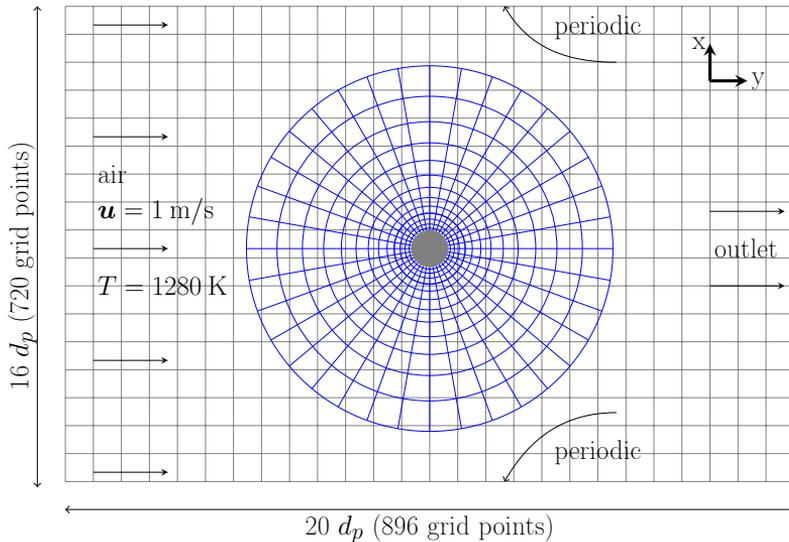
Figure 5: Schematic representation of the analyzed case (not drawn to scale)
