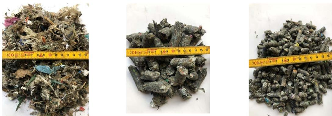
Figure 3: SRF waste. Loose form (left); 16 mm pellets (mid); 8 mm pellets (right).
