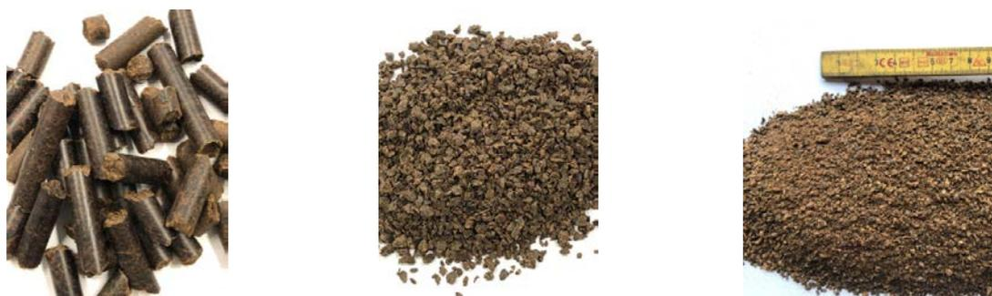
Figure 2: Wood pellets. 8 mm pellets (left); milled and sieved > 800 μm (mid); milled and un-sieved (right).
