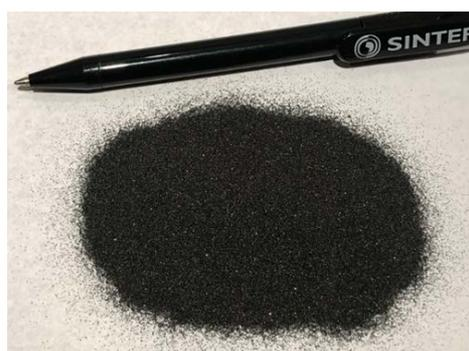
Figure 4: Sample of ilmenite 120 – 200  $\mu\text{m}$ .
