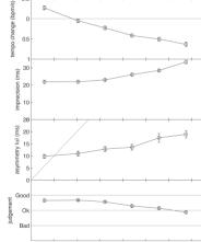
The tempo increased for the 6 ms delay but decreased for delays of 21 ms and longer.
