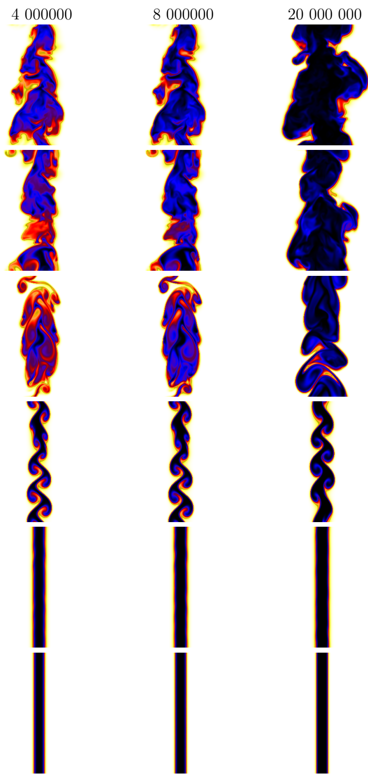
Figure 21: Figure shows snapshots for reactant flow for density 10^4 \text{kg}/\text{m}^3 for different particles amount
