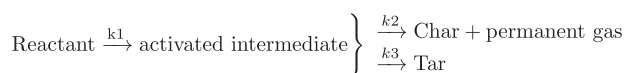
Fig. 10. Broido–Shafizadeh scheme. This reaction model assumes the formation of an intermediate that eventually forms the final products char, permanent gas and tar.
