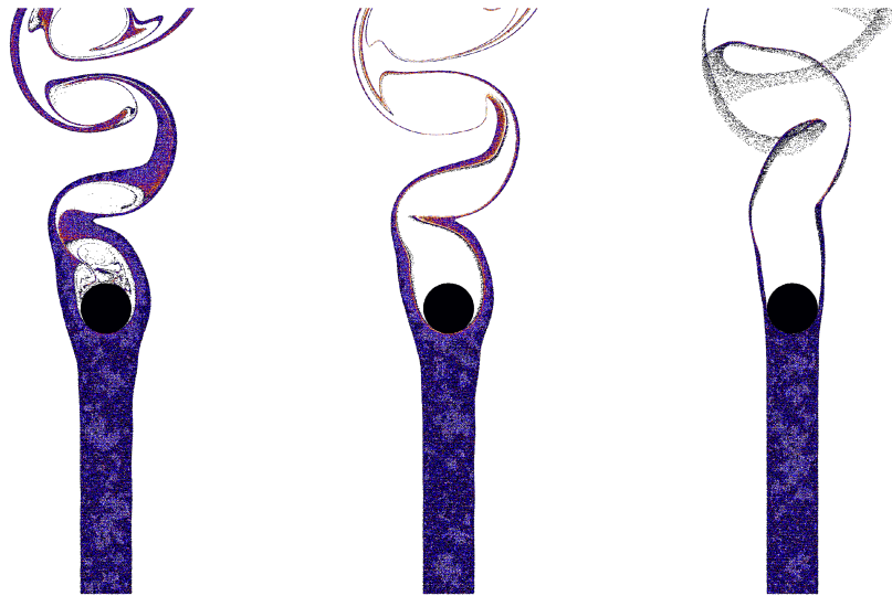
Figure 3: Snapshot of particle number density for simulation with Re = 1600 , and Stokes number of 0.08 (left), 0.3 (middle) and 10 (right). Grid resolution for this simulation was 2048 \times 1024 grid points.
