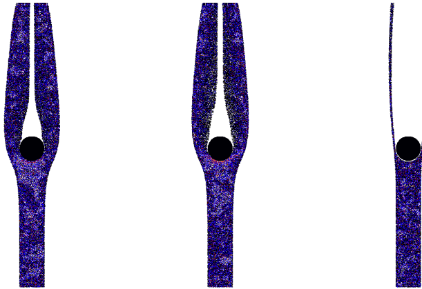
Figure 1: Snapshot of particle number per grid cell for simulation with Re = 20 , and Stokes number of 0.08 (left), 0.3 (middle) and 10 (right). Grid resolution for this simulation was 1024 \times 512 grid points. The relation between color coding and number of particles pr. grid cell is the following: 0 particles; white, 1 particle; black, 2 particles; blue, 3 particles; red, 4 particles; orange 5 or more particles; yellow.
