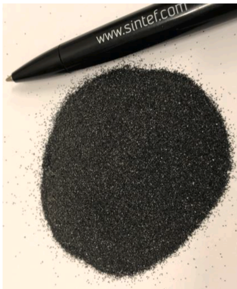
Fig. 6. Sample of ilmenite 150 – 350 \mu\text{m} .
