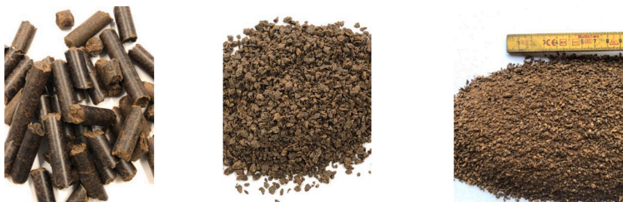
Fig. 4. Wood pellets. 8 mm pellets; milled and sieved; milled and un-sieved (left to right).
